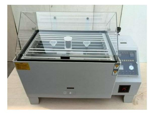
The Salt Spray Chamber are specialized to test the performance of the products for its surface of various materials after treatment of corrosive protection by means of painting, coating, galvanizing, anodizing and of lubricant.
